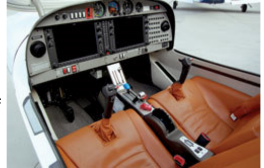
The cabin of the DA40 XLS features a sports car-like interior with a center-stick design that appears to grow out of the seats
