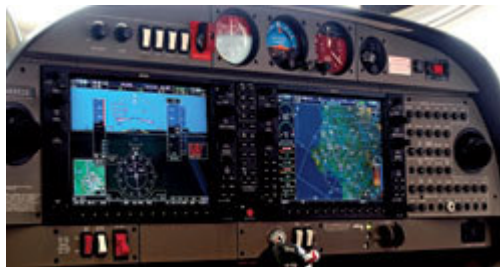
The aircraft is equipped with Garmin's G1000 glass panel, and Synthetic Vision Technology offers a 3-D view of surrounding terrain and potential obstacles.
